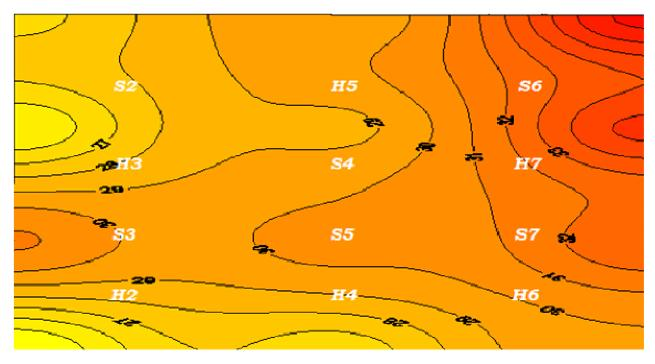
Figure 5. Temperature map inside the greenhouse on July 29, 2007 at 02:00 p.m.
