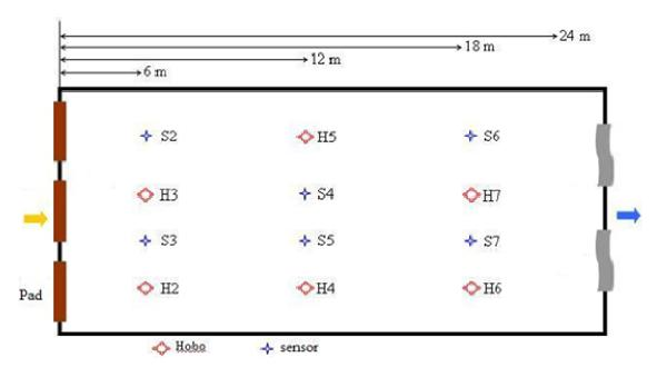
Figure 1. The location of sensors in the greenhouse.
