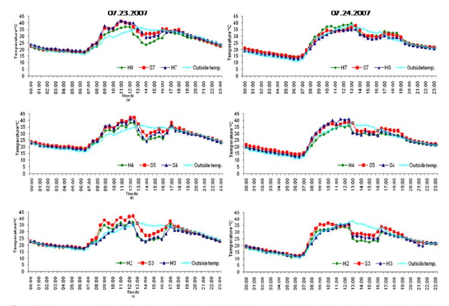
Figure 2. Hourly temperature variations as indicated by sensors (a) in front of the fan, (b) in the center line, (c) in front of the pad, on July 23, 2007 and on July 24, 2007.
