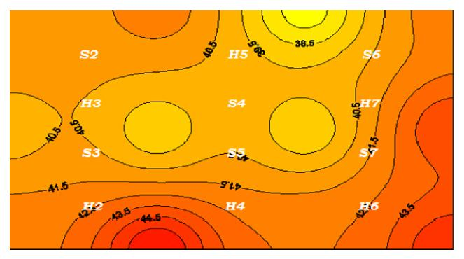
Figure 4. The temperature map inside the greenhouse on July 28, 2007 at 02:00 p.m. when the system was not operating.
