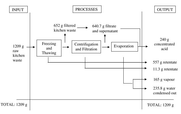
Figure 5. Material balance for the recovery of organic acids from fermented kitchen waste.
