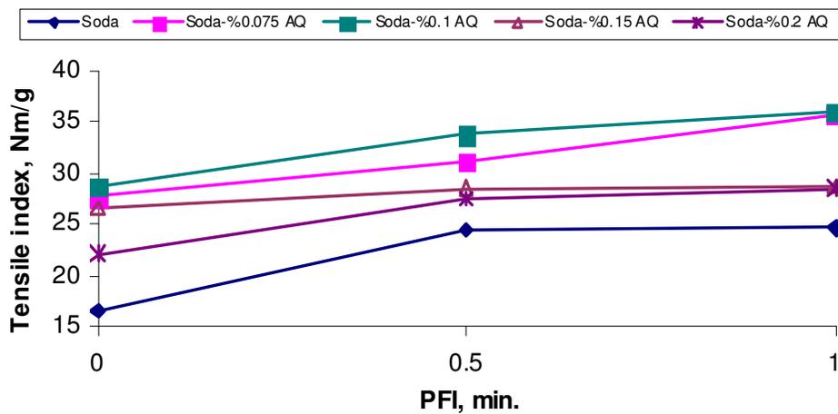
Figure 3. Effect of AQ on tensile strength.
