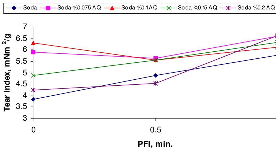
Figure 5. Effect of AQ on tear strength.
