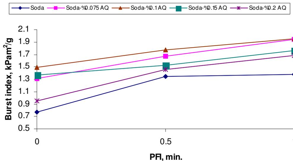
Figure 4. Effect of AQ on burst strength.
