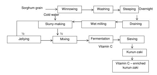
Figure 1. The modified laboratory method of kunun-zaki production (Egbere et al, 2008).
