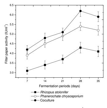
**Figure 5.** Filter paper enzyme activity (IU ml<sup>-1</sup>) of coirwaste substrate and supplemented with urea substrate during solid state fermentation with *R. stolonifer, P. chrysosporium* and coculture. Mean  $\pm$  S.E indicated. The filter paper activity significantly at probability level (P < 0.05).
