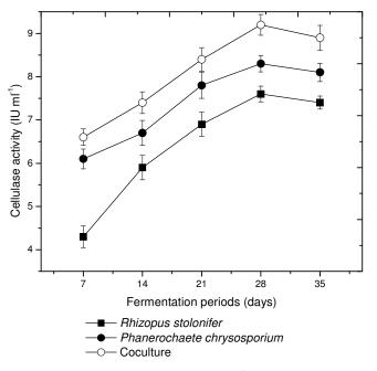
**Figure 4.** Cellulase enzyme activity (IU ml<sup>-1</sup>) of coirwaste substrate and supplemented with urea substrate during solid state fermentation with *R. stolonifer, P. chrysosporium* and coculture. Mean  $\pm$  S.E indicated. The cellulase activity significantly at probability level (P < 0.05).
