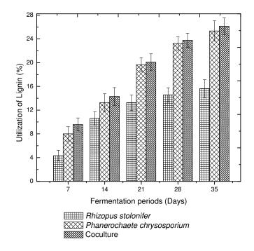
**Figure 1.** Utilization of lignin (%) in coirwaste substrate during solid state fermentation with *R. stolonifer, P. chrysosporium* and coculture. Mean  $\pm$  S.E indicated. The lignin conversion was significantly at probability level (P < 0.05).
