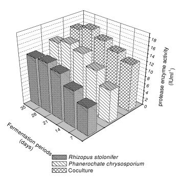
**Figure 8.** Protease enzyme activity (IU ml<sup>-1</sup>) of coirwaste substrate and supplemented with urea substrate during solid state fermentation with *R. stolonifer, P. chrysosporium* and coculture. Mean  $\pm$  S.E indicated. The protease enzyme activity significantly at probability level (P < 0.05).
