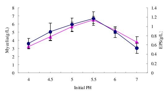
**Figure 1.** Effect of initial pH on the mycelial growth and exopolysaccharide production by *Hirsutella* sp. in shake-flask culture: (•) the concentration of exopolysaccharide and ( $\blacktriangle$ ) mycelial dry weight.
