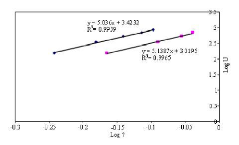
**Figure** 8. Linear regression plot of Richardson-Zaki correlation. Linear regression plot of the Richardson-Zaki correlation as described by Equation 8 were demonstrated on the acetate binding buffer pH 5 ( $\bullet$ ) and 4.5 % (w/v) wet biomass unclarified feedstock ( $\blacksquare$ ). Richardson-Zaki coefficient (n) obtained from the slope of logarithm of superficial velocity (log U) versus logarithm of bed voidage (log  $\epsilon$ ).
