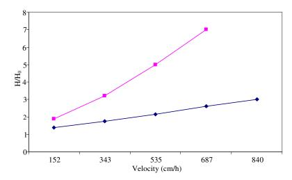
**Figure** 7. Bed expansion characteristic. Bed expansion characteristic of STREAMLINE Direct HST adsorbent by acetate binding buffer pH 5 ( $\blacklozenge$ ) and 4.5% (w/v) wet biomass unclarified feedstock ( $\blacksquare$ ). H denoted expanded bed height and H<sub>0</sub> denoted settled bed height.
