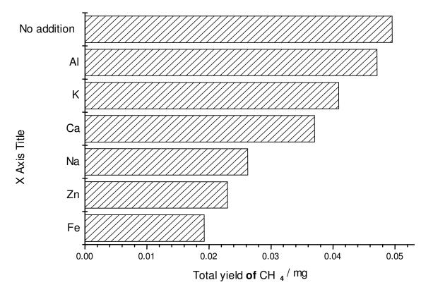
Figure 6. Effect of metal addition on the total yield of CH<sub>4</sub>.
