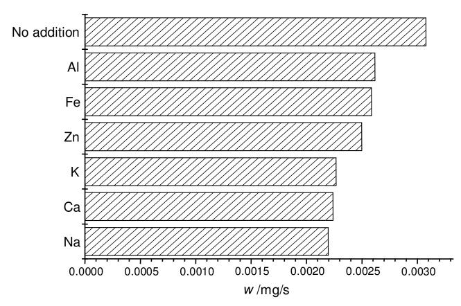
Figure 7. Effect of metal addition on the reaction rate of sawdust pyrolysis.
