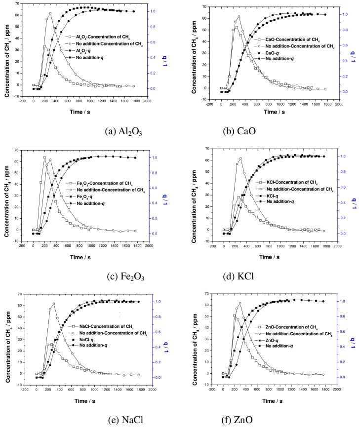
Figure 5. Effect of metal addition on the evolution of CH4.
