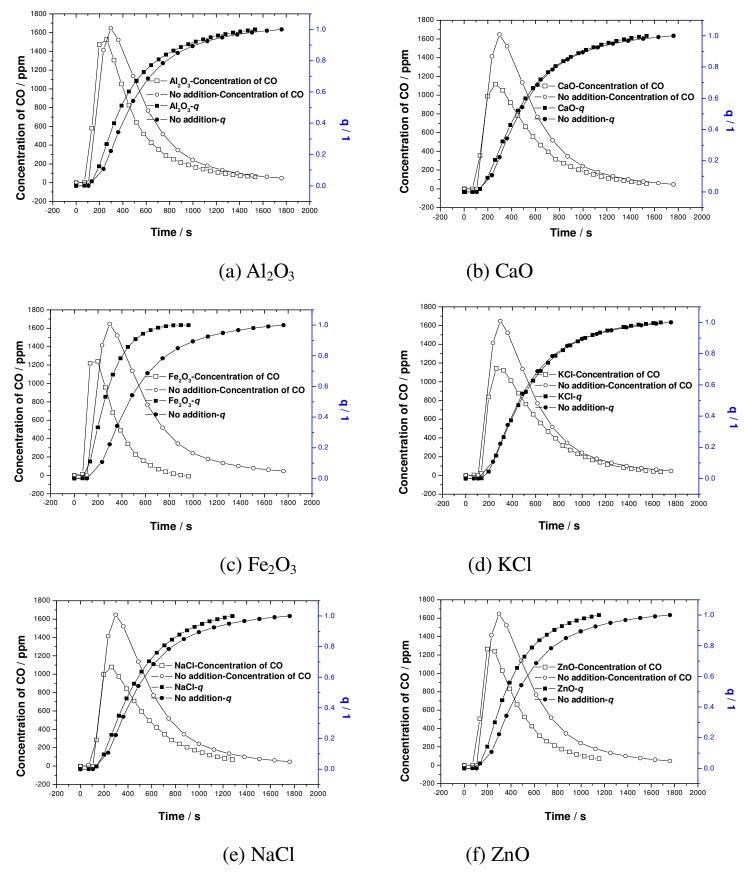
Figure 3. Effect of metal addition on the evolution of CO.
