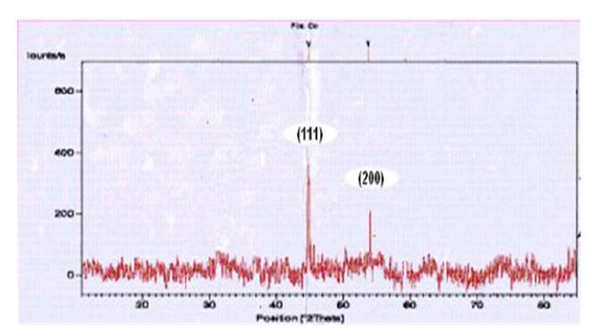
Figure 5. X-ray diffraction patterns of Co nano particles.
