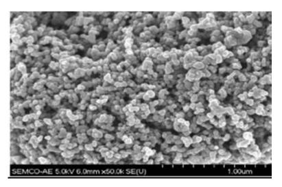
Figure 4. SEM of Co-nano particles.
