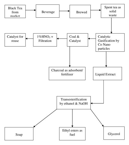
Figure 1. Schematic representation of the biofuel production from spent tea.
