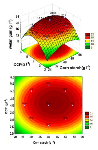
**Figure 2.** 3D response surface and 2D contour plots showing interaction between corn starch concentration and CCF concentration on the production of welan gum.
