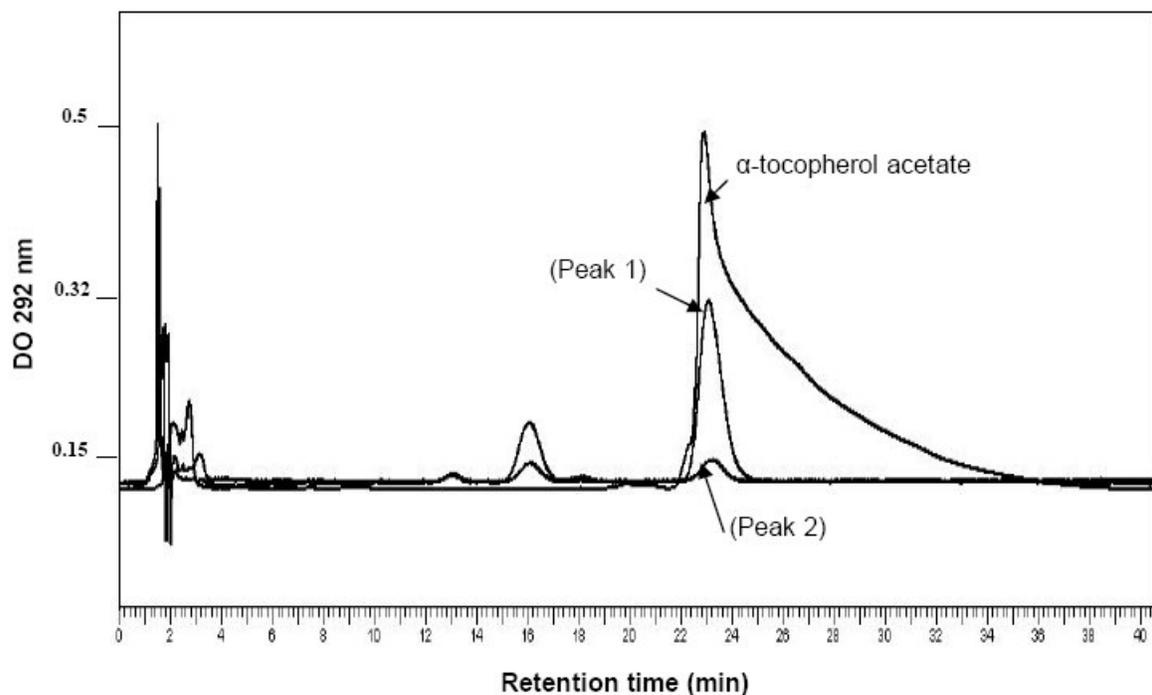
**Figure 2.** C18-HPLC chromatogram of  $\alpha$ -tocopherol acetate (supplemented vitamin E) (23 min). Fat of animals fed with 200 mg vitamin E/kg of food (23 min) (peak 1) and fat of control animals fed only with the basal diet (25 mg vitamin E/kg of food) (25 min) (peak 2). Injected sample volume was 100  $\mu$ l of fat solution. Elution was performed with methanol/water solution at 1.5 ml/min and the absorbance of eluted fractions was measured at 292 nm.
