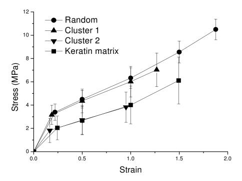
Figure 5. Tensile responses of neat keratin and composites.
