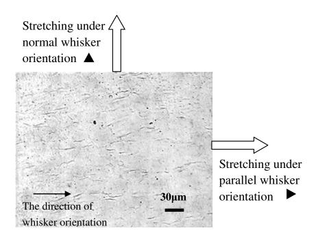
Figure 6. Sketch of whisker orientation in matrix.
