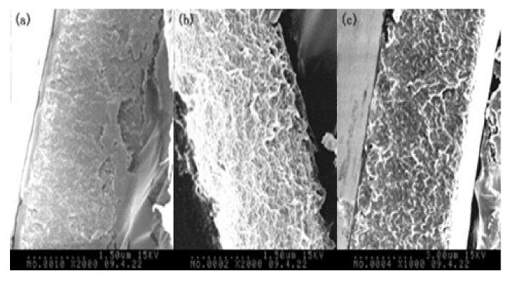
Figure 8. (a) SEM morphology of neat keratin, (b) no coupled composite reinforced by whiskers, and (c) coupled composite and whisker orient randomly.
