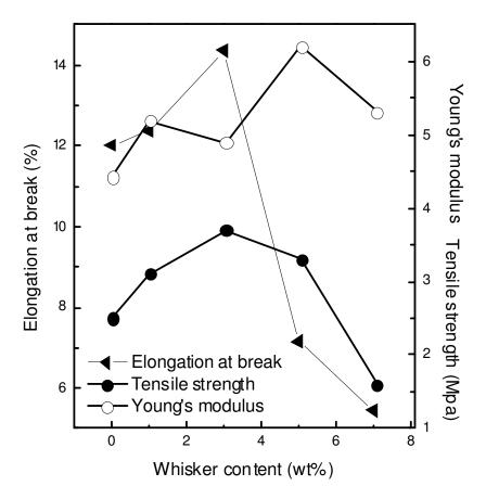
Figure 3. The elongation at break, tensile strength and Young's modulus of composites with various whisker contents.
