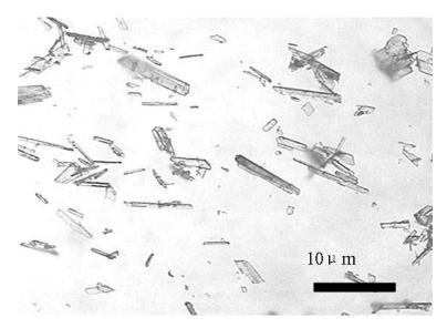
Figure 1. Optical micrograph of K<sub>2</sub>Ti<sub>6</sub>O<sub>13</sub> whiskers.
