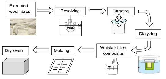
Figure 2. Schematic diagram of the whiskers reinforced membranes fabrication.
