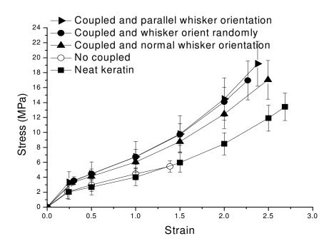
Figure 7. Tensile responses of neat keratin and composites.
