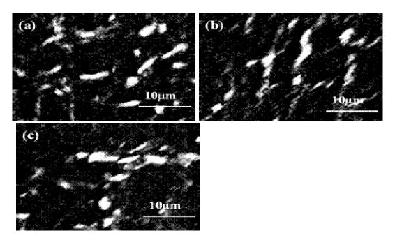
**Figure 4.** Micrographs of whiskers reinforced keratin films: (a) random whiskers distribution, (b) whiskers cluster microstructure (cluster 1) and (c) whiskers cluster microstructure (cluster 2).
