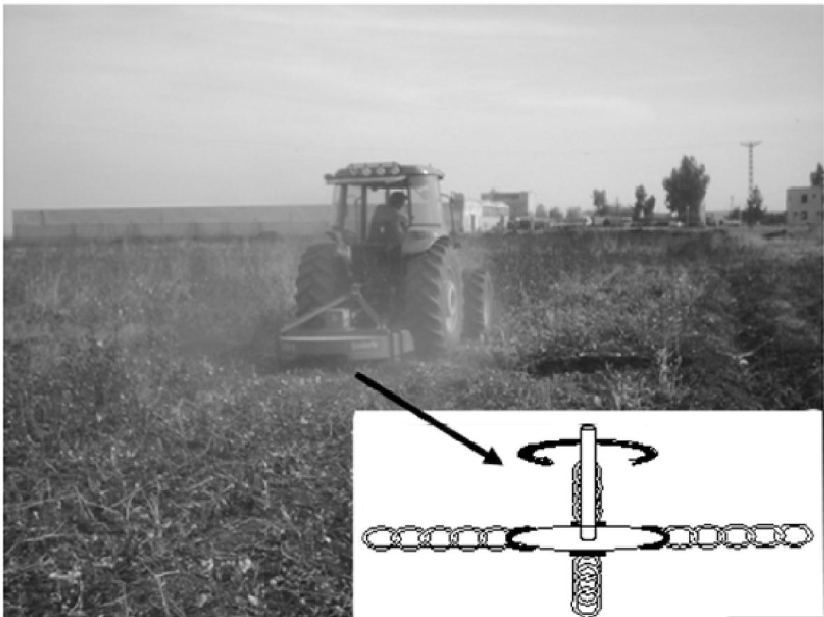
**Figure 3.** Chained-type stalk chopper.
