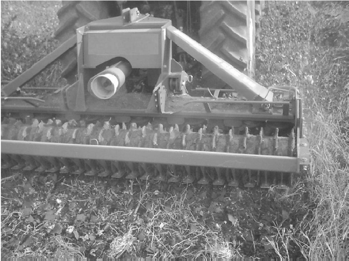
**Figure 4.** Vertical-blade rotating dredge.
