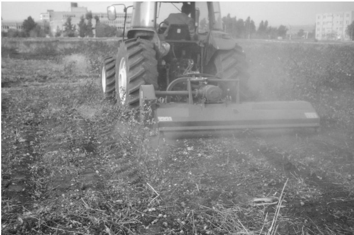
**Figure 1.** Splined-type stalk chopper.
