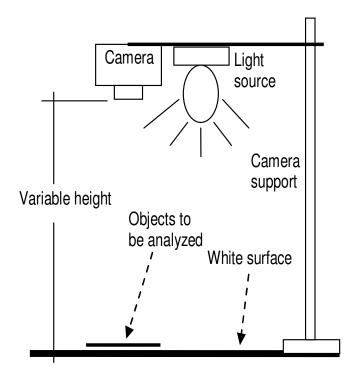
Figure 1. Camera set up.
