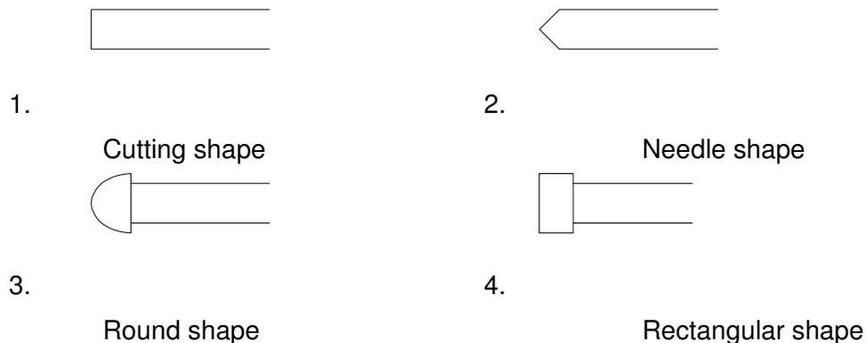
**Figure 2.** Type of electrodes use in ozonizer; 1) cutting shape, 2) needle shape, 3) round shape, and 4) rectangular shape.
