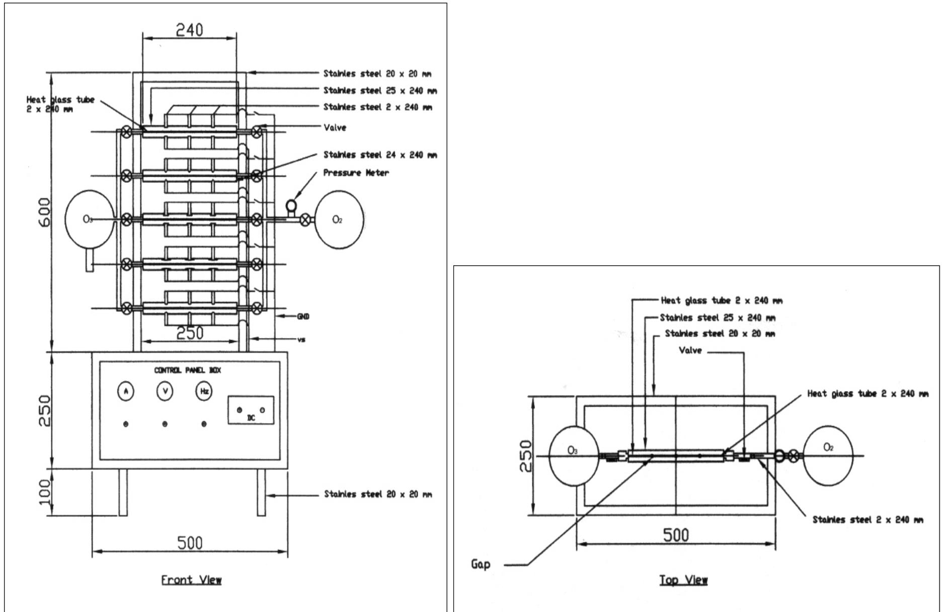
Figure 1. Schematic diagram of a pilot scale ozonizer.
