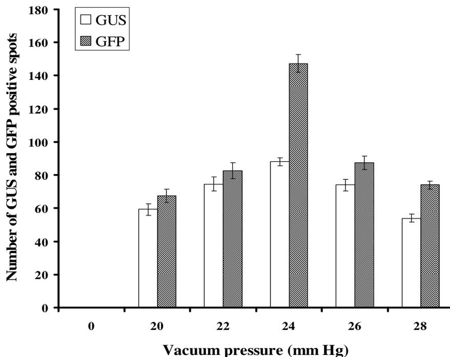
**Figure 4.** Effect of vacuum pressure on transient gene expression of GFP and GUS genes in *A. donax* using biolistic device-gene gun
