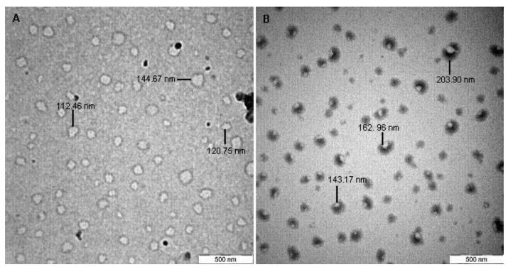
Figure 1. Transmission electron micrograph of nanostructured lipid carriers. (A) NLC80 and (B) NLC20.
