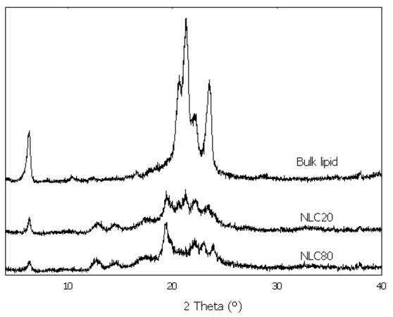
Figure 4. X-ray diffraction pattern of lipid bulk material; NLC20 and NLC80.
