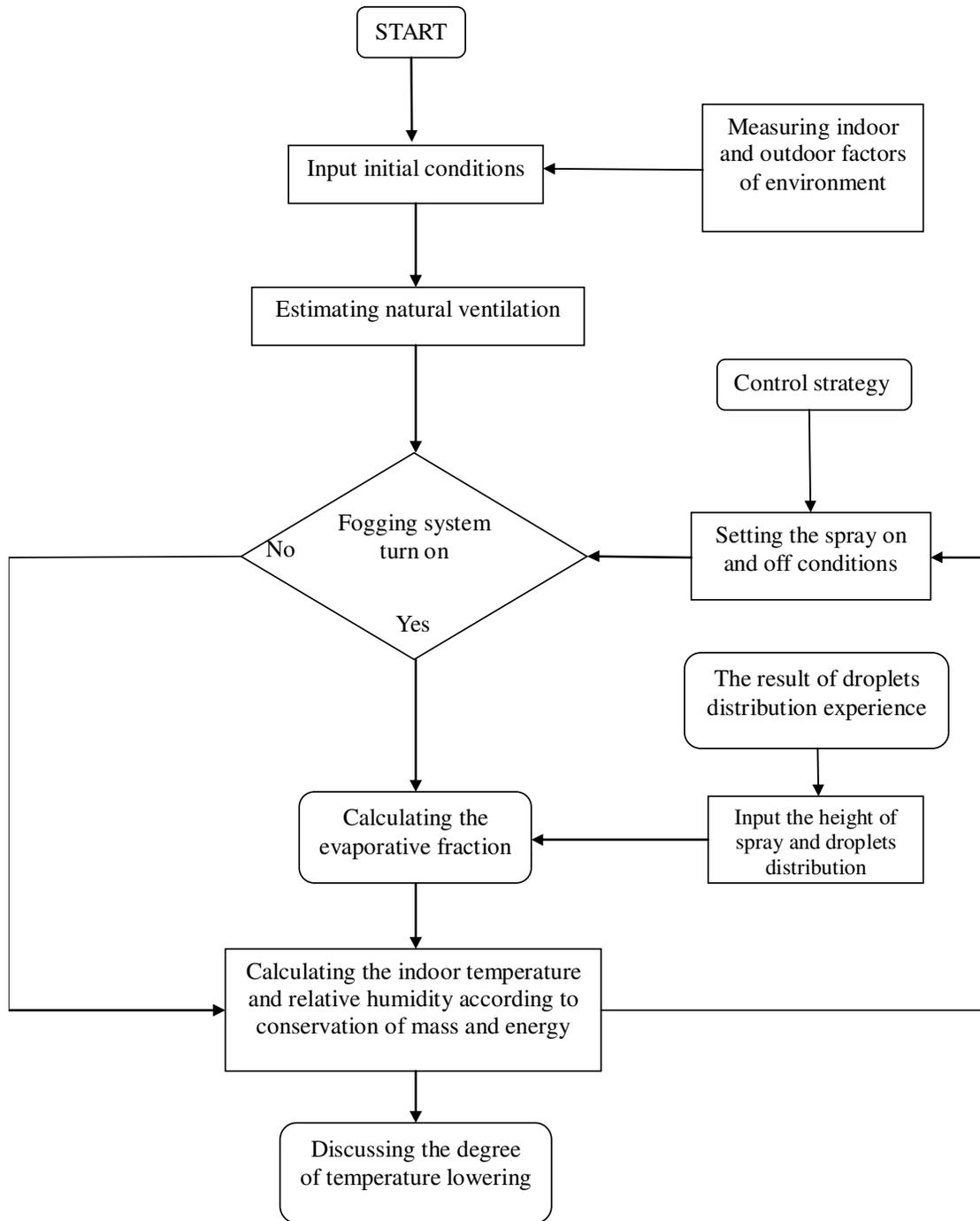
Figure 1. Flowchart showing the simulation procedure.
