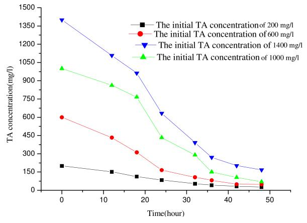
Figure 4. The degradation curve of the TA concentration.
