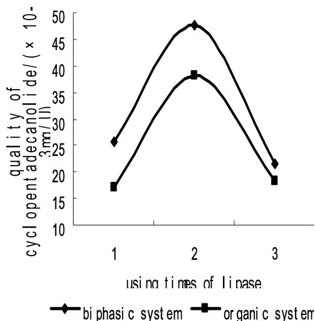
**Figure 7.** Effect of CSL GXU08 reusability on the production of cyclopentadecanolide under the same conditions of  $T=40^{\circ}\text{C}$ ,  $C_{\text{substrate}} = 8 \text{ mmol/l}$ ,  $\omega=180 \text{ r/min}$ ,  $\text{pH}= 6.5$  and  $t= 72 \text{ h}$ . Data presented are mean values with deviation of less than 5%.
