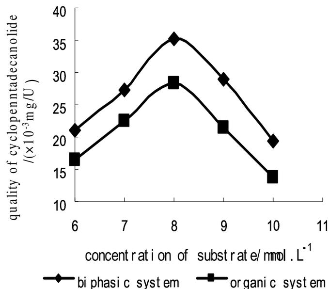
**Figure 5.** Effect of concentration of substrates on the production of cyclopentadecanolide under the same conditions of  $T=40^{\circ}\text{C}$ ,  $\text{pH}=7.0$ ,  $\omega=180$  r/min and  $t=72$  h. Data presented are mean values with deviation of less than 5%.
