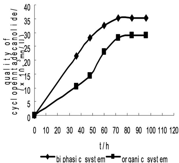
**Figure 3.** Effect of reaction time on the production of cyclopentadecanolide under the same conditions of T= 40°C, pH= 7.0,  $\omega=180$  r/min. Data presented are mean values with deviation of less than 5%.
