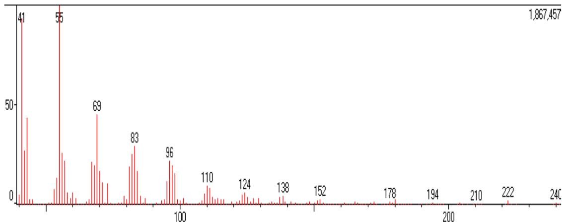
**Figure 1.** The mass spectrum of cyclopentadecanolide sample at retain time  $t = 11.703$  min in gas chromatography.
