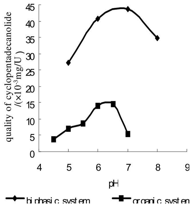
**Figure 6.** Effect of pH on the production of cyclopentadecanolide under the same conditions of  $T=40^{\circ}\text{C}$ ,  $C_{\text{SUB}}=8$  mmol/l,  $\omega=180$  r/min and  $t=72$  h. Data presented are mean values with deviation of less than 5%.
