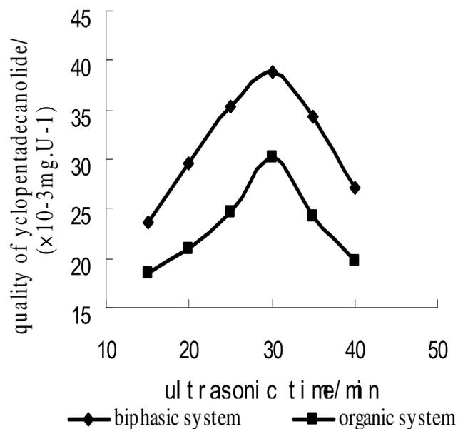
**Figure 8.** Effect of ultrasonic time on reaction.
