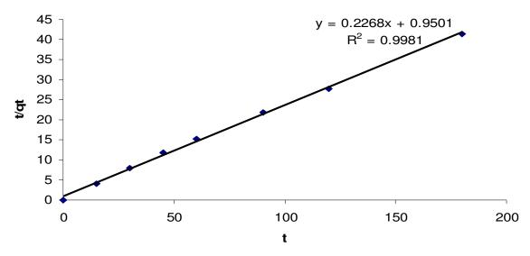
**Figure 7.** Pseudo 2<sup>nd</sup> order kinetic model for Foron Turquoise SBLN dye removal by *G. lucidum* and *C. versicolor* biomass.
