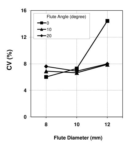
Figure 2. The CV values obtained from flute helical angle and flute diameter combination.
