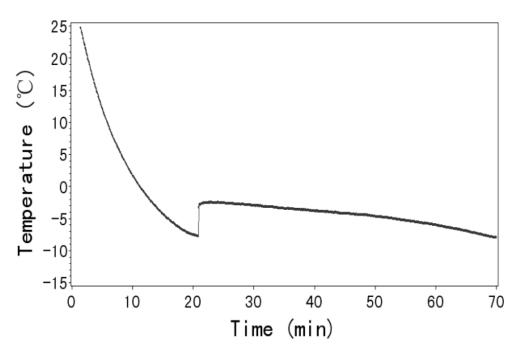
Figure 1. A typical freezing curves of sweet corn kernel.
