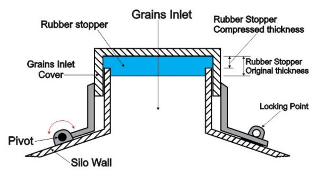
**Figure 3.** Section view of rubber stopper compressed in-between silo grain inlet cover and silo top edge of grain inlet opening. The same techniques can be applied to the discharge lid for achieving hermitical sealing.
