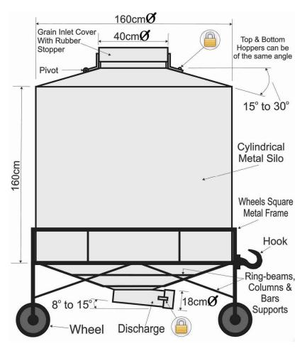
Figure 1. Side view of the cylindrical mobile metal silo.
