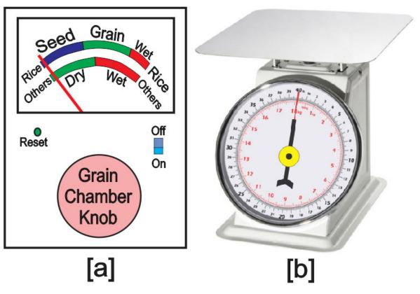
**Figure 4.** (a) Grains moisture tester diagram; If the needle-pointer is in the Blue range means the grain is ≤12% moisture content. If the pointer is in the Green range, the grain is 12 to 14% moisture content, if the pointer is at Red range, the grain is too wet to store. (b) Table dial weighing scale for testing grain weight.
