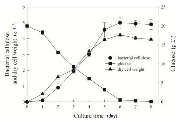
**Figure 2.** Time course of BC production by the isolated *Gluconacetobacter* sp. RKY5 under a static culture condition at 30°C in 250 ml Erlenmeyer flask containing 50 ml of HS medium.
