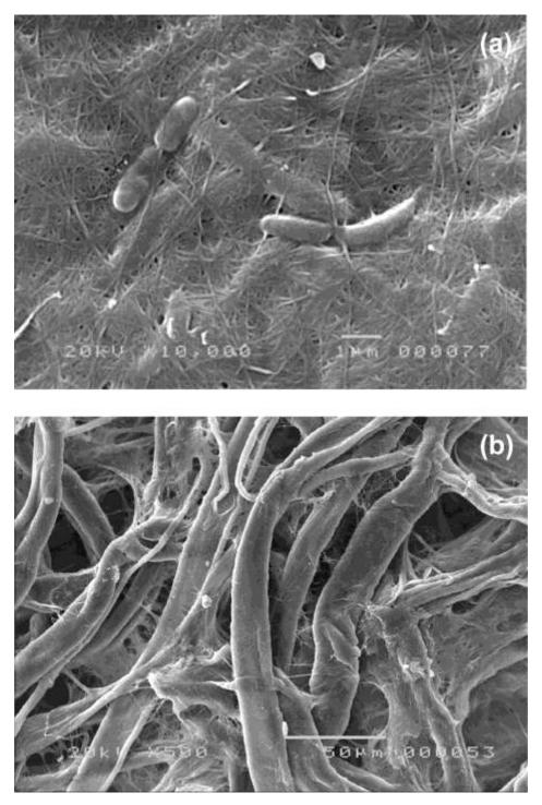
**Figure 3.** Scanning electron micrograph of (a) BC produced by *Gluconacetobacter* sp. RKY5 and (b) filter paper. The elliptical mass shown in (a) is the cells of *Gluconacetobacter* sp. RKY5 embedded in the BC.
