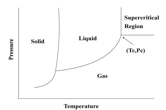
Figure 1. Small changes in temperature and pressure near the critical region will affect the density and solubility of SCFs.
