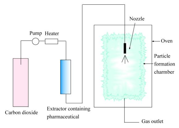
Figure 2. The equipment commonly used in RESS.
