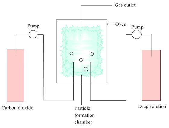
Figure 3. The equipment commonly used in GAS.
