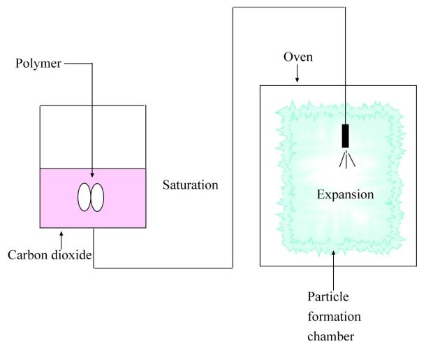
Figure 4. The equipment commonly used in PGSS.
