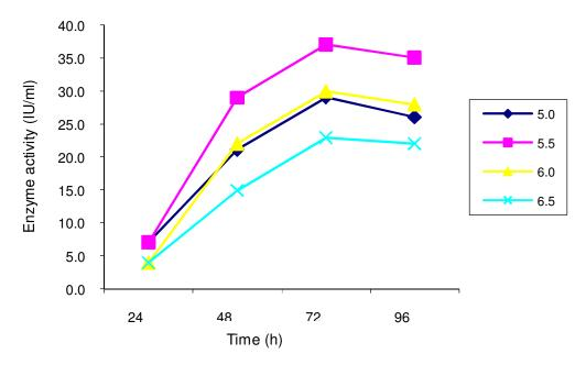
**Figure 2.** Xylanase production by *A. niger* during 96 h fermentation at  $27.5 \,^{\circ}$ C and  $2.5 \,^{\circ}$ c orn cobs concentration in culture medium at different pH levels.
