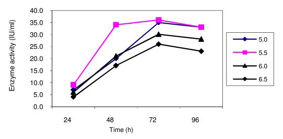
**Figure 12.** Xylanase production by A. *niger* during 96 h fermentation at 32.5 ℃ and 3.5% corn cobs in culture medium at different pH levels.
