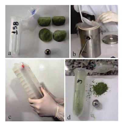
**Figure 1.** Proposed cacao leaf maceration protocol: a) tube, steel spheres and 15-mm leaf disks; b) freezing the tubes containing the spheres and the leaf discs lyophilized in liquid nitrogen; c) manual agitation of a set of samples; d) fine powder obtained.
