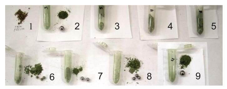
**Figure 3.** Parameters tested to optimize the maceration process ranging between: type of tissue, quantity of spheres, number of leaf disks and size of sphere (mm), respectively. 1 = fresh, 1, 4 and 6; 2 = lyophilized, 1, 3 and 6; 3 = fresh, 1, 5 and 4; 4 = fresh, 1, 4 and 3; 5 = fresh, 1, 6 and 2; 6 = lyophilized, 3, 4 and 2; 7 = lyophilized, 2, 4 and 5; 8 = lyophilized, 3, 4 and 3; 9 = lyophilized, 1, 4 and 6.
