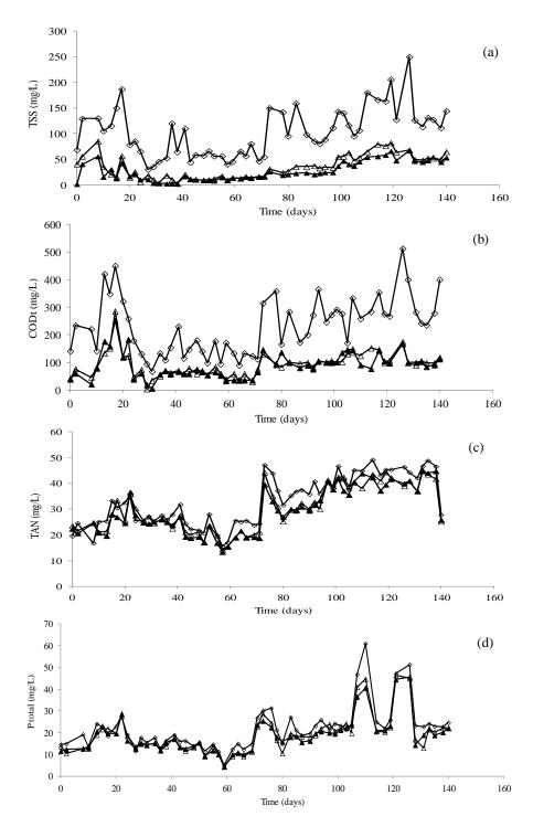
**Figure 5.** Concentrations of (a) the total suspended solids (TSS), (b) the total chemical oxygen demand (COD<sub>t</sub>), (c) the total Ammonium nitrogen (TAN) and (d) the total phosphorous ( $P_{total}$ ) in the Influent ( $\Diamond$ ), ACF1 Effluent ( $\Delta$ ) and ACF2 Effluent ( $\blacktriangle$ ) during the entire study period.
