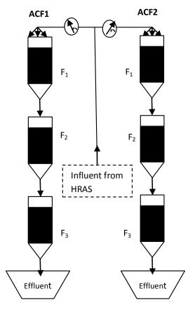
**Figure 3.** Schematic representation of the setup of the alternating charcoal filter 1 (ACF1) with a retention time of 2.5 h and the alternating charcoal filters 2 (ACF2) with a retention time of 5 h.
