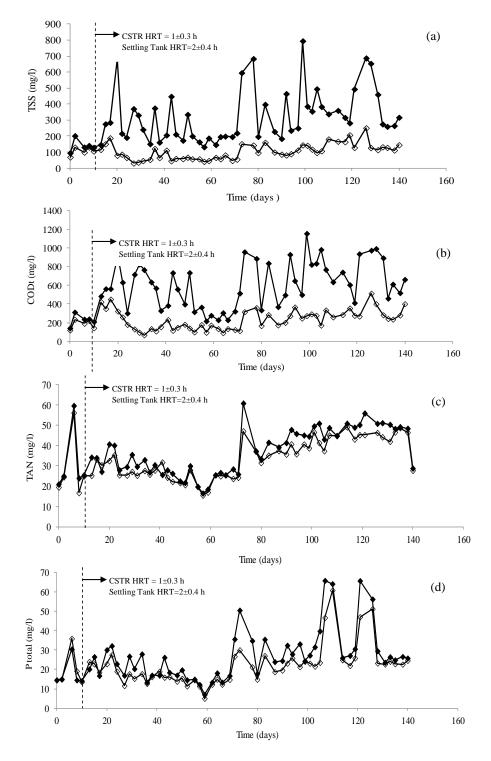
**Figure 4.** Influent ( $\blacklozenge$ ) and effluent ( $\diamondsuit$ ) concentrations of (a) the total suspended solids (TSS), (b) the total chemical oxygen demand (COD<sub>t</sub>), (c) the total Ammonium nitrogen (TAN) and (d) the total phosphorous (P<sub>total</sub>), in the high rate activated sludge system during the entire study period.
