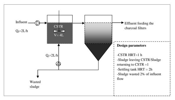
Figure 2. Schematic representation of the high-rate activated sludge (HRAS) set-up consisting of a completely mixed reactor (CSTR) in series with a settler.
