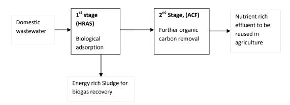
**Figure 1.** Representation of the combined processes treatment with use of high rate activated sludge (HRAS) system and the alternating charcoal filter (ACF).
