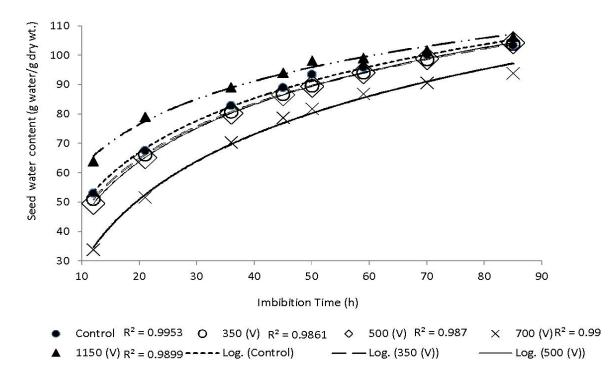
Figure 1. Logarithmic trend between water uptake (percentage) and imbibition time for different voltages at the fixed temperatures 17.5°C.
