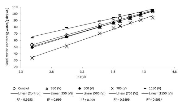
Figure 2. Linear increase between water uptake (%) and logarithm of time (h) for different voltages at the fixed temperatures 17.5°C.
