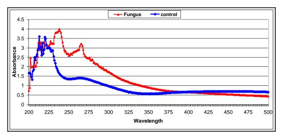
Figure 1. UV-Vis spectra of iron nanoparticles biologically synthesized by fungus.
