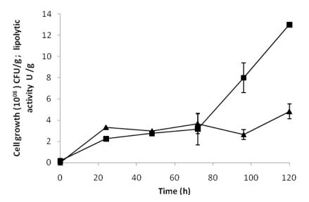
**Figure 4.** Production of lipase and biomass in SSF for 120h at 30°C; (▲) Lipolytic activity; (■) Cell viability.
