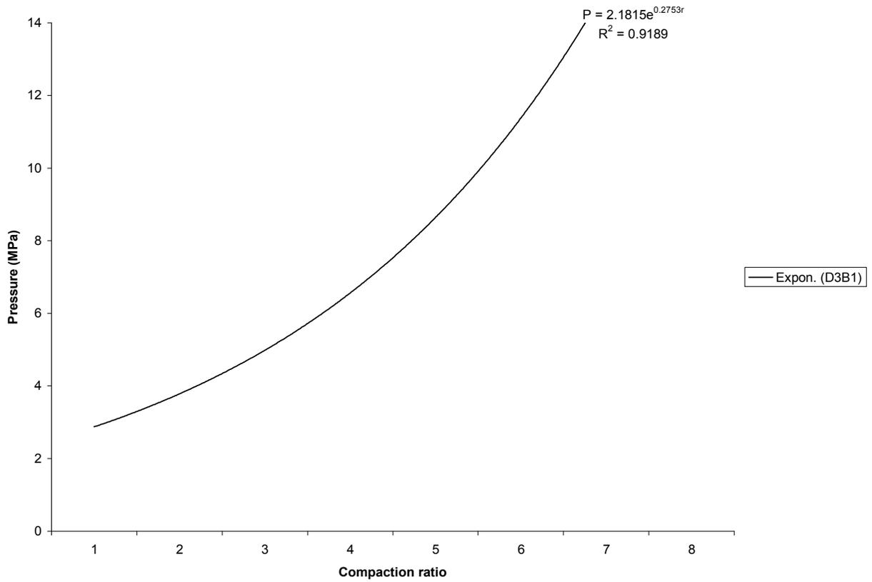
Figure 5. Relationship between pressure and compaction ratio for D<sub>3</sub>B<sub>1</sub>.
