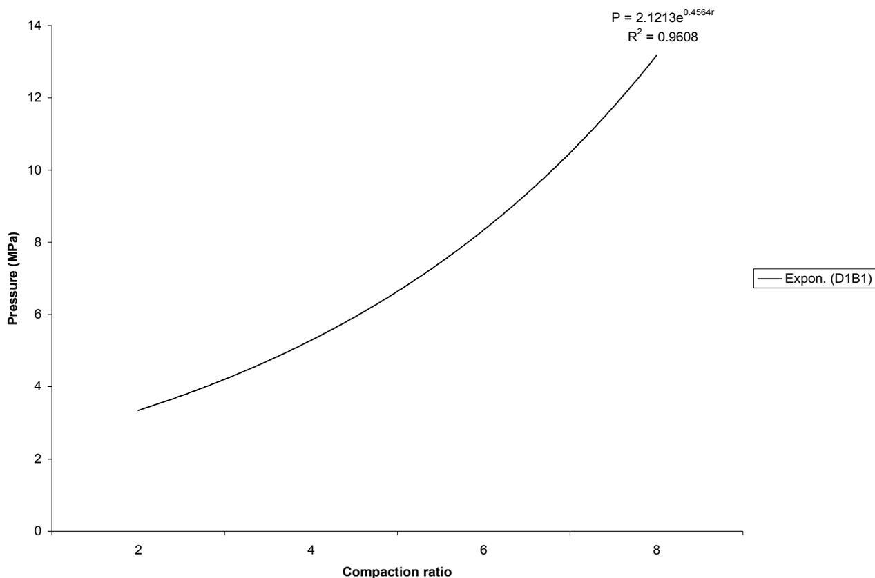
**Figure 3.** Relationship between pressure and compaction ratio for D<sub>1</sub>B<sub>1</sub>.
