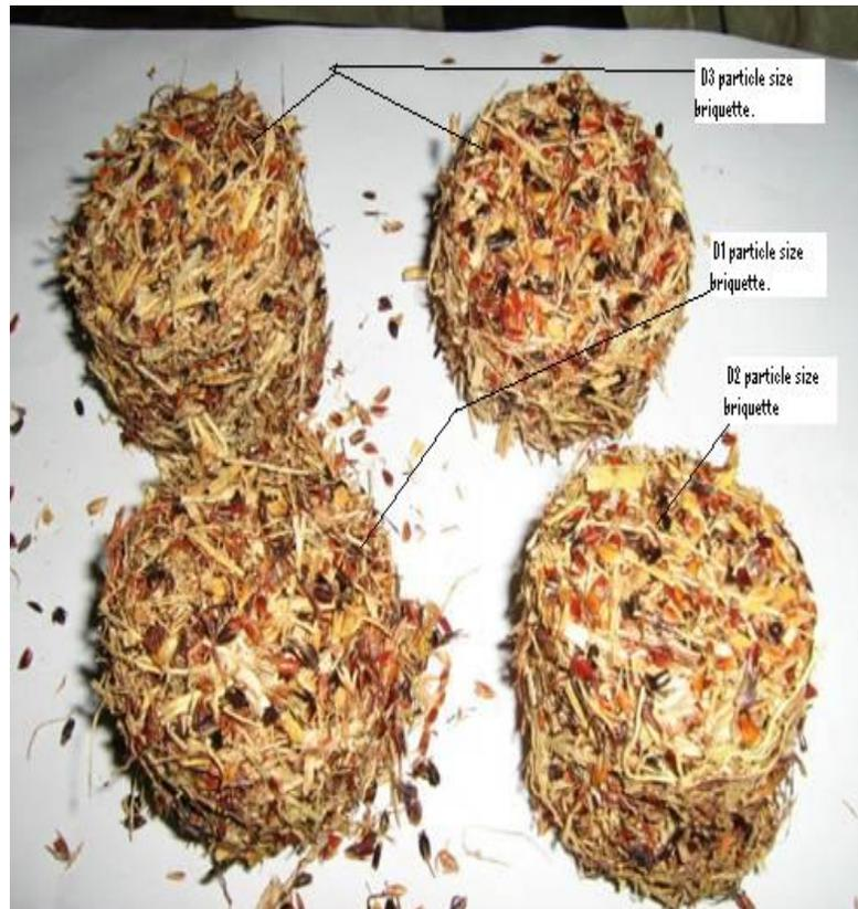
Figure 2. Briquettes produced form the hydraulic press.
