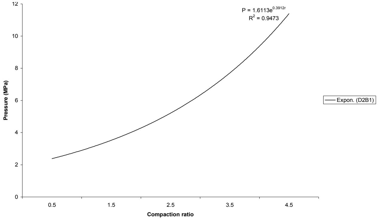
Figure 4. Relationship between pressure and compaction ratio for D<sub>2</sub>B<sub>1</sub>.
