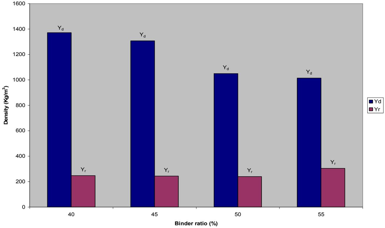
Figure 8. Effect of binder ratio on maximum and relaxed density for D<sub>1</sub> particle size briquettes.
