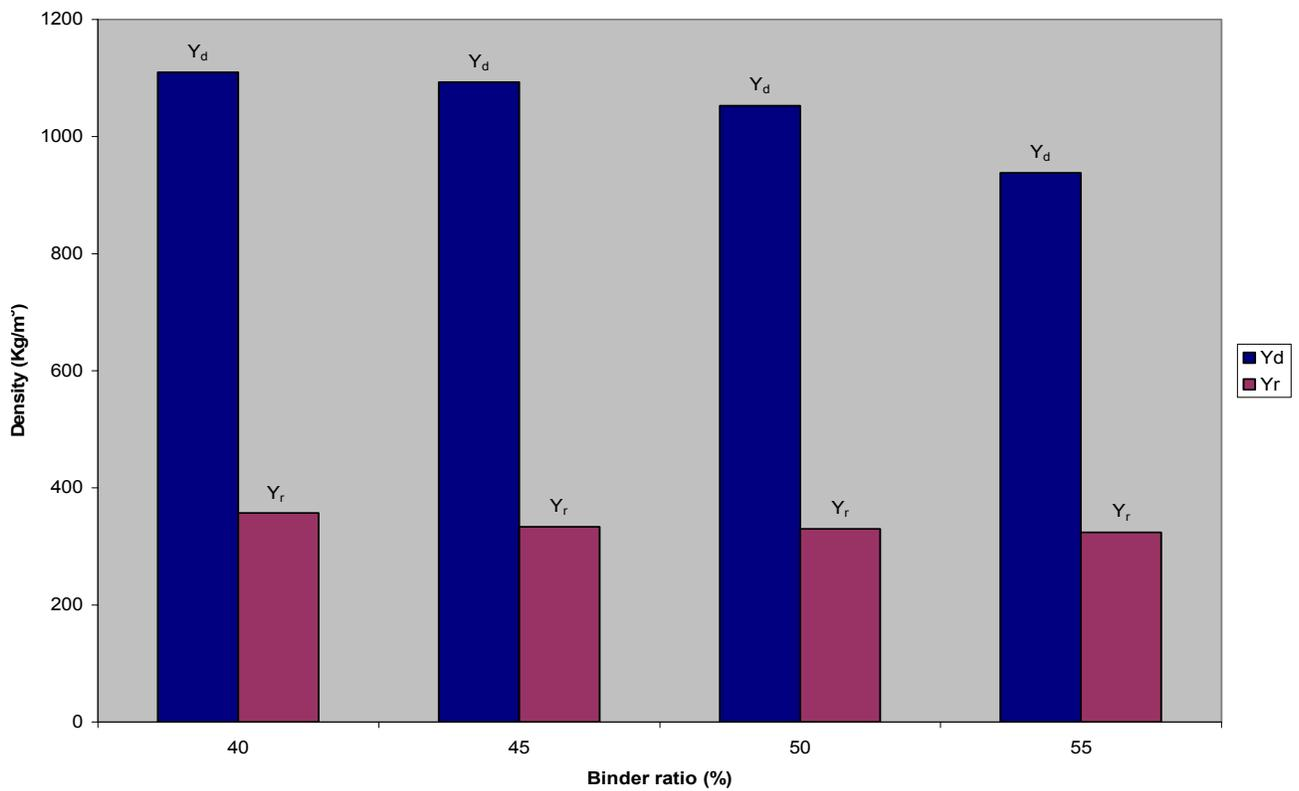
Figure 9. Effect of binder ratio on maximum and relaxed density for D<sub>2</sub> particle size briquettes.
