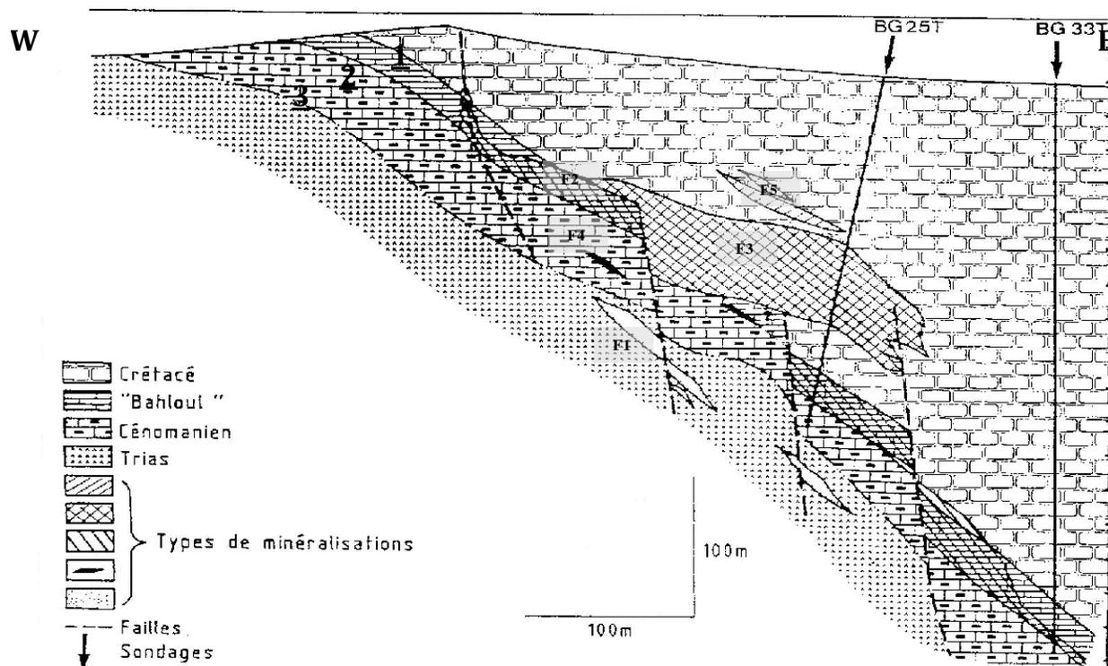
**Figure 1.** Schematic section W-E of Bougrine mining (Orgeval, 1986). Geological levels: 1, Cenomanian Turonian; 2, basic Cenomanian; 3, transition zone Triassic/Cretaceous.
