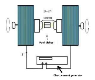
**Figure 1.** The experimental electromagnet apparatus. Three Petri dishes are placed in the air gap between the two iron bars to expose the seeds to the static magnetic field.
