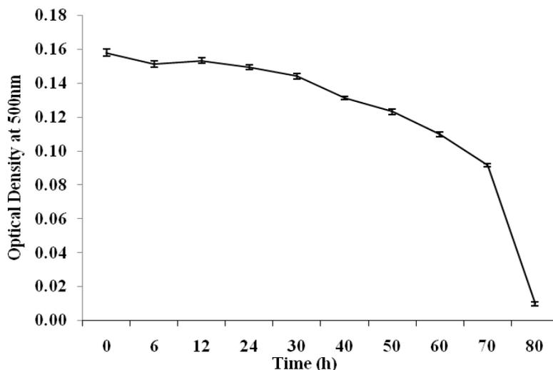
**Figure 1.** Time-course of phenol degradation of MSG8 in liquid MSM containing 9.5 mM phenol initially. The results are shown as average of six independent experiments and the bars indicate the standard deviation less than 5%.
