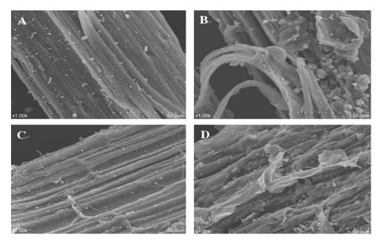
**Figure 5.** SEM of rice straw and corn stalk samples. Rice straw before enzymatic hydrolysis (A), corn stalk before enzymatic hydrolysis (B); rice straw after enzymatic hydrolysis (C) and corn stalk (D). SignalName=SE, accelerating voltage=20000 volt, Deceleration voltage=0 v, Magnification=1000, working reistance=9400 um, Emission current=50000 nA.
