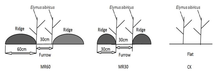
Figure 2. The schematic diagram presenting the three different systems in the study.
