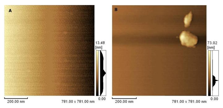
Figure 1. AFM images of mica surface (a) and zinc oxide nanopartcles (b).
