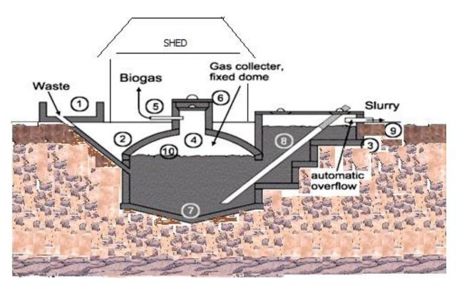
**Figure 2.** Fixed dome plant Nicarao design. 1. Mixing tank with inlet pipe and sand trap. 2. Digester. 3. compensation and removal tank. 4. Gas holder. 5. Gas pipe. 6. Entry hatch, with gastight seal. 7. Accumulation of thick sludge. 8. Outlet pipe. 9. Reference level. 10. Supernatant scum, broken up by varying level (GTZ, 1999).
