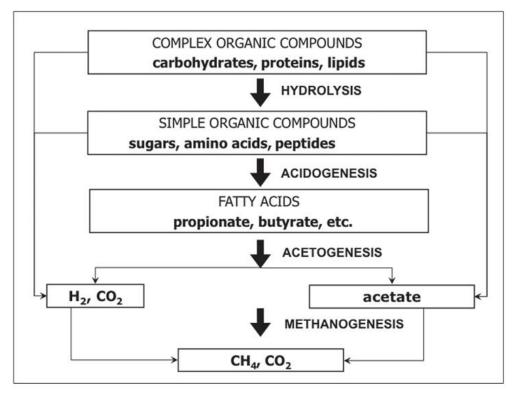
**Figure 1.** Simplified schematic representation of the anaerobic degradation process (Lettinga et al., 1999).
