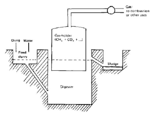
Figure 3. Floating-drum plant.
