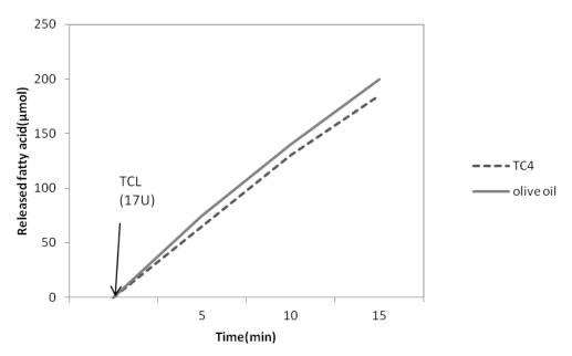
**Figure 3.** Kinetic of hydrolysis of olive oil or tributyrin emulsions by TCL (17 U). Lipolytic activity was followed at pH 8 and 50°C.
