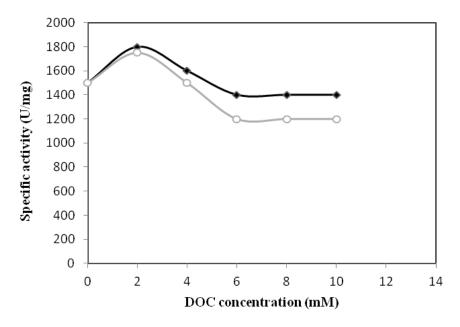
**Figure 5.** Effect of increasing concentration of NaDC on the rate of hydrolysis of tributyrin (○) and olive oil emulsion (◆) by TCL.lipolytic activity was measured under standard conditions at pH 8 and 50°C using a pH-stat.
