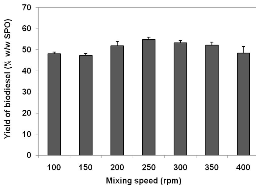
**Figure 6.** Effect of mixing speed on biodiesel production from sludge palm oil (SPO) using locally produced *Candida cylindracea* lipase.
