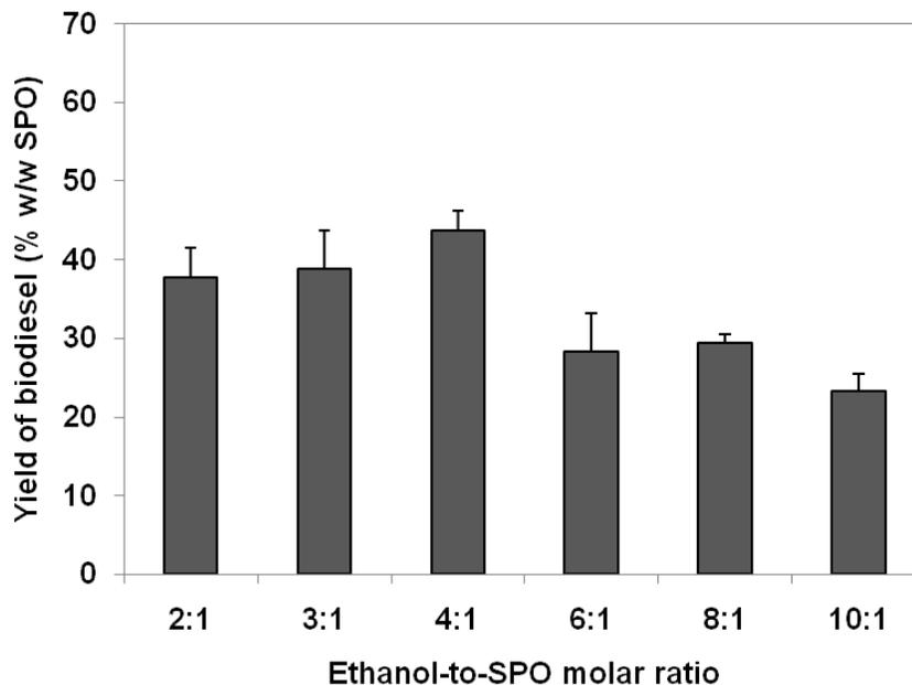
**Figure 3.** Effect of ethanol-to-SPO molar ratio on biodiesel production from sludge palm oil (SPO) using locally produced *Candida cylindracea* lipase.
