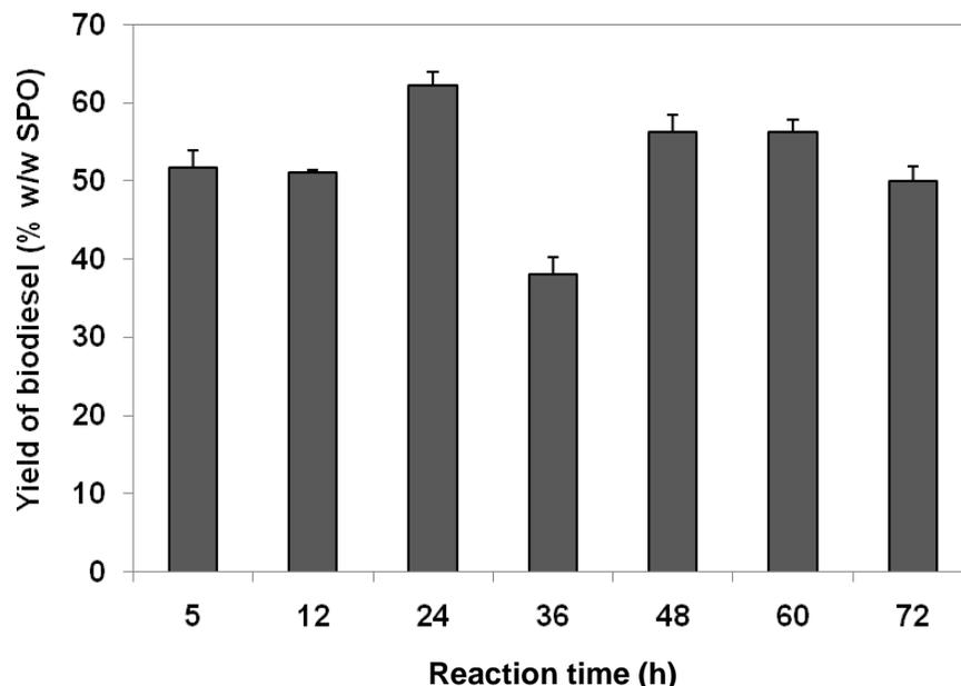
**Figure 7.** Effect of reaction time on biodiesel production from sludge palm oil (SPO) using locally produced *Candida cylindracea* lipase.
