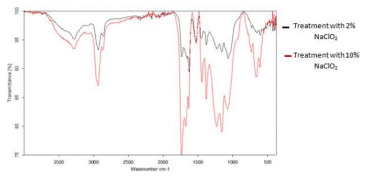
Figure 3. Cellulose FT-IR spectrum extracted from N. gaditama by 2% NaOH followed by 6 and 10% of NaClO2.
