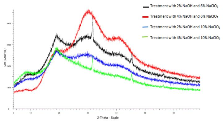
Figure 4. X-ray diffractogram of cellulose extracted from 2 and 4% of NaOH followed by bleaching 6 and 10% of NaClO<sub>2</sub>
