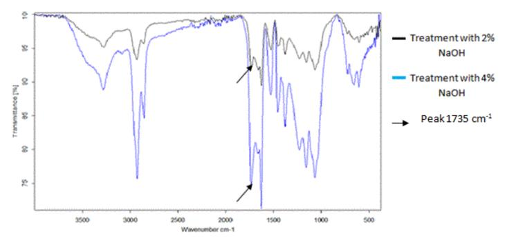
Figure 2. Cellulose FT-IR spectrum extracted from N. gaditama by 2 and 4% NaOH followed by 10% of NaClO2.
