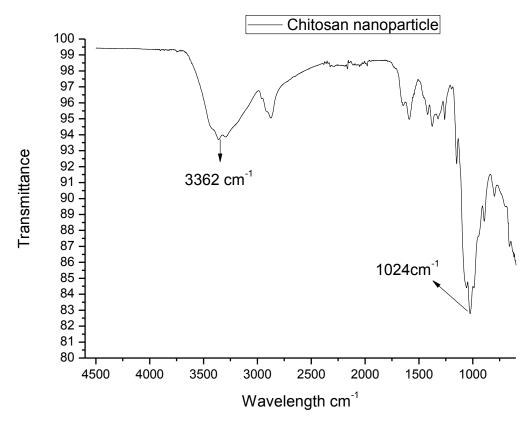
Figure 2. Chitosan nanoparticle spectrum in the FTIR.
