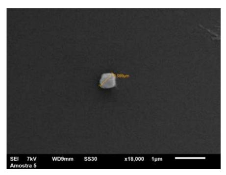
Figure 8. Nanoparticles produced from spray-dry system by gelation method NaOH.
