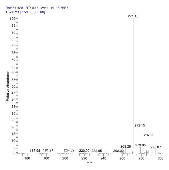
Figure 2. ESI-MS spectrum for estrone.
