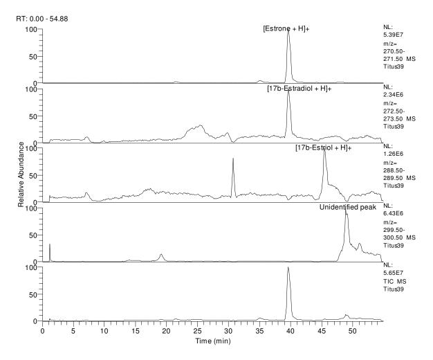
Figure 3. SLM/LC-ESI-SIM-MS of a mixture of estradiols in milk. Mobile phase contained 75% 25 mM acetic acid at concentrations 0.1  $\mu$ g/L.
