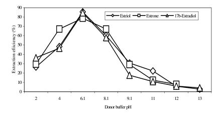
**Figure 1.** Donor optimization in the extraction of  $17\beta$ -estradiol and its metabolites: Membrane = di-n-hexyl ether:n-undecane (1:1) with 5% TOPO; extraction time = 60 min, flow rate = 0.1 ml/min; acceptor solution = Na<sub>2</sub>HPO<sub>4</sub>/NaOH, pH 13.
