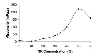
**Figure 2.** Effect of NR concentration on the viscosity of methylol Urea (formaldehyde/urea mole ratio = 3:1, temperature =  $70^{\circ}$ C, time = 2 h).
