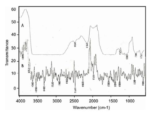
Figure 1. IR spectra of MUR (A) and MUR-NR composite (B).
