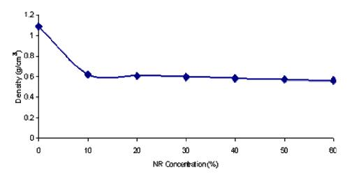
Figure 4. Effect of NR concentration on the density of methylol urea (formaldehyde/urea mole ratio = 3:1, temperature =  $70^{\circ}$ C, time = 2 h).
