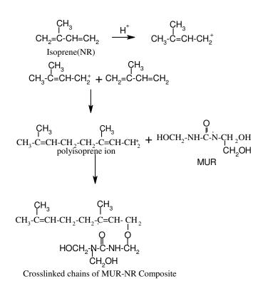
(i) Between two methylol groups or between one methylol group and active hydrogen atoms of the composite as indicated below:
