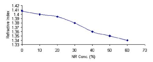
Figure 3. Effect of NR concentration on refractive index of methylol urea (formaldehyde/urea mole ratio = 3:1, temperature =  $70^{\circ}$ C, time = 2 h.
