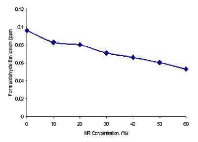
**Figure 5.** Effect of NR concentration on the formaldehyde emission of methylol urea (formaldehyde/urea mole ratio = 3:1, temperature =  $70^{\circ}$ C, time = 2 h).
