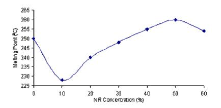
**Figure 6.** Effect of NR concentration on the melting point of methylol urea (formaldehyde/urea mole ratio = 3:1, temperature =  $70^{\circ}$ C, time = 2 h).
