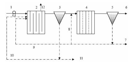
**Figure 1.** The schematic diagram of pilot-scale experiment: (1) influent; (2) anaerobic baffled reactor(ABR, composed of Compartment I-VI); (3) settling tank; (4) Plug Flow Reactor (PFR, composed of Compartment I-VI); (5) settling tank; (6) effluent; (7) discharged aerobic excess sludge; (8) recycling aerobic sludge to PFR; (9) recycling aerobic sludge to ABR; (10) recycling anaerobic sludge to ABR; (11) discharged anaerobic excess sludge; (12) biogas.
