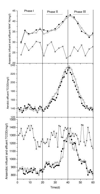
**Figure 2.** Experimental performances of system A and B. Aerobic excess sludge recirculation ratio for system A: Phase I (1 - 20 d): 60%; Phase II (21 - 40 d): 70%; Phase III (41 - 60 d): 60%. Ratio of system B: Phase I: 40%; Phase II: 50%; Phase III: 40%. Note: "—\*— Influent, —•— System A (SRT: 10 d), —•— System B (SRT: 25 d)"
