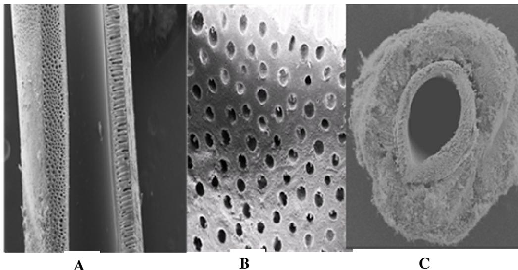
**Figure 1.** (A) SEM of a longitudinal section of the polysulphone membrane. (B) The external surface of the polysulphone membrane showing cavities where spores can be immobilised. (C) *P. chrysosporium* biofilm immobilised on the external surface of the polysulphone membrane.
