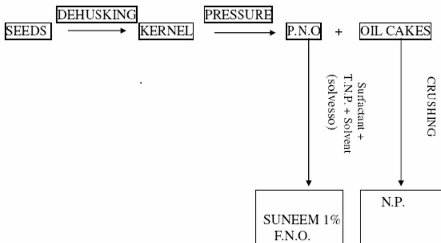
**Figure 1.** Process to obtain the neem products (*Azadirachta indica*, A. Juss) (Provided by the SENCHIM chemistry's industry Dakar- SENEGAL). P.N.O., pure neem oil; F.N.O., formulated neem oil; T.N.P., technical neem powder; and N.P., neem powder.
