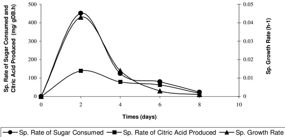
**Figure 4.** Specific rate data showing microbial growth, sugar consumption and citric acid production on TRBS in solid state flask fermentation.
