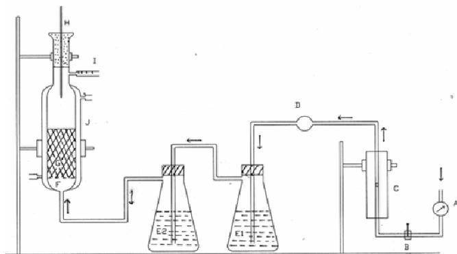
**Figure 1.** Schematic diagram showing packed bed bioreactor set up. A = Compressor, B = Gate Valve, C = Rotameter, D = PTFE Air Filter, E1 & E2 = Humidifying Bottles, F = Perforated Plate, G = Column Reactor, H = Beckman's Thermometer, I = Glass Wool Air Filter For Outlet of Exhaust Air, and J = Jacketed Wall of Reactor.
