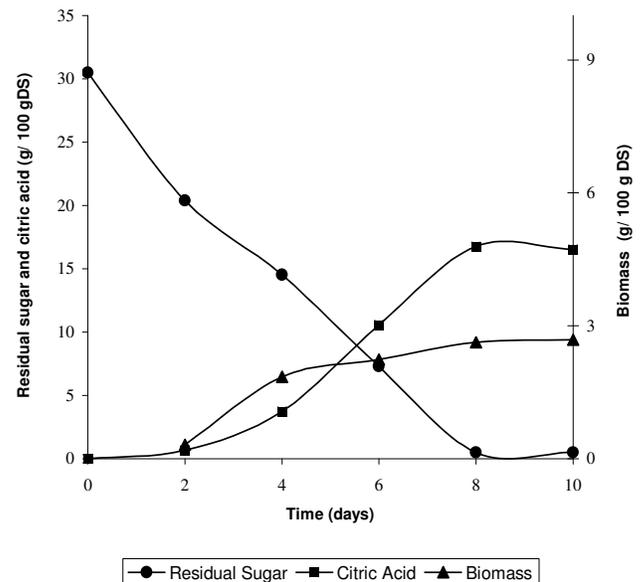
**Figure 6.** Microbial growth and citric acid production on TRBS in packed bed reactor.
